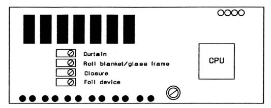
Potentiometer for the setting of the run-down current Spin direction for the motor run-down setting:
